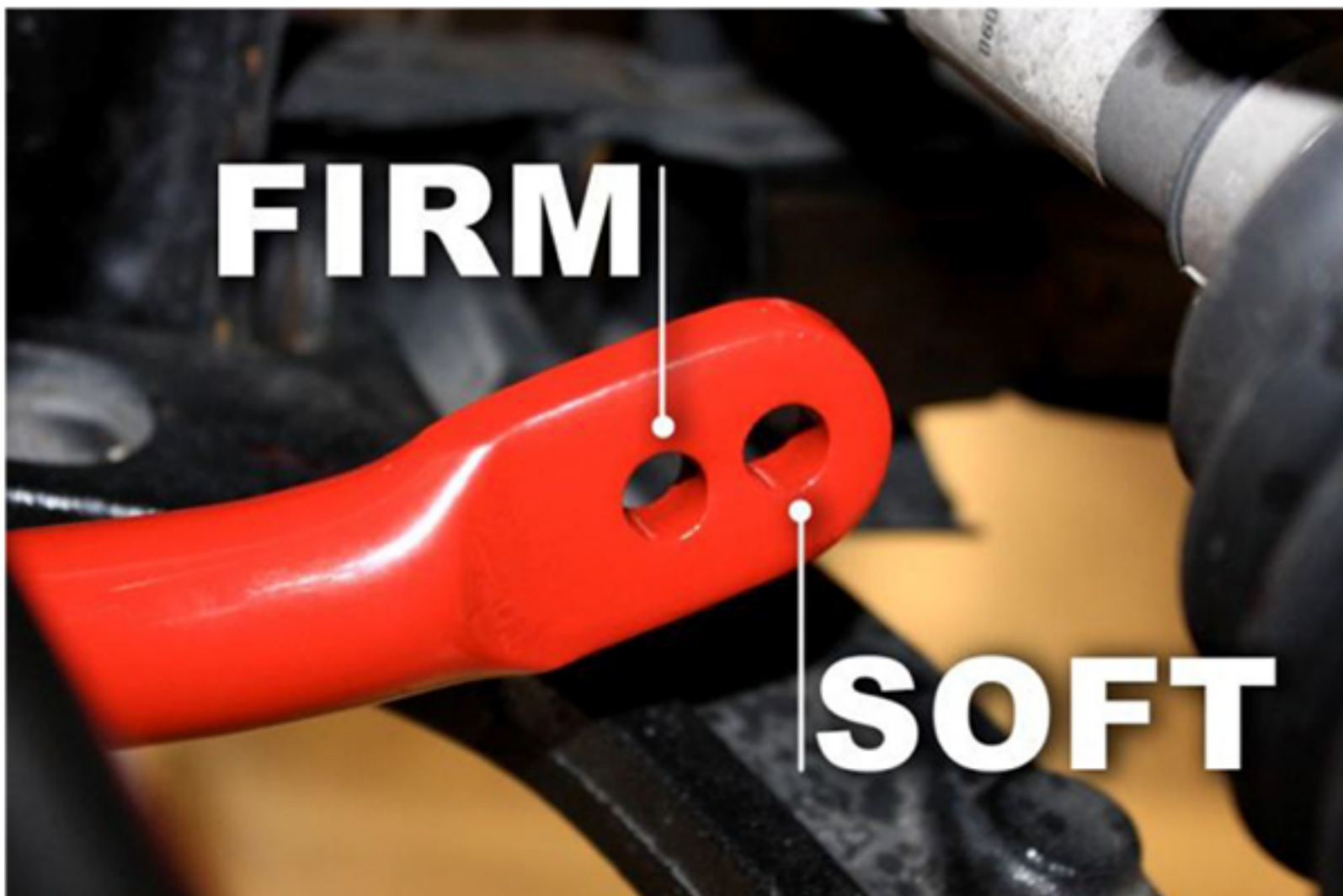
16. Hole adjustment positions. See Adjustment Chart.
