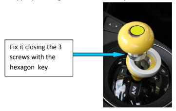
6. Reassembly the knob by turning the lower part. Place the ring with the BLACK name, if present, in the proper location.
