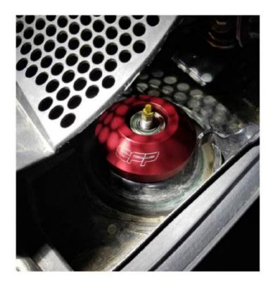
Note: It is important that you insure that you have at least 3-4 threads minimum protruding above the bearing.
