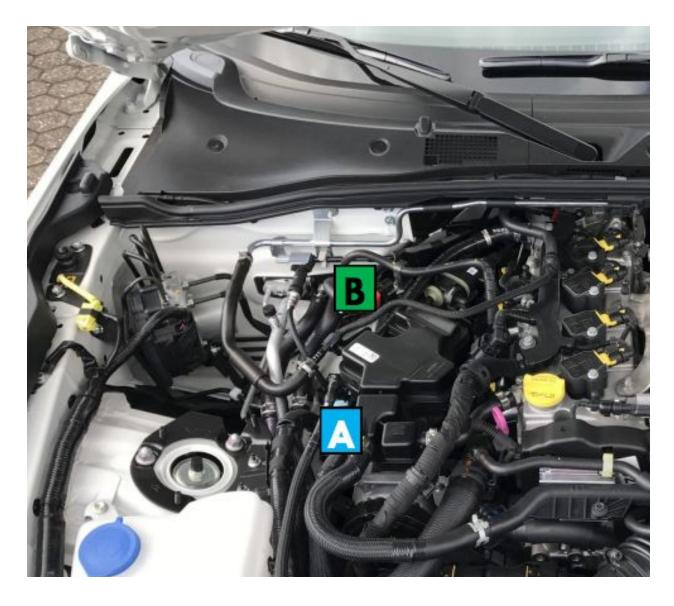
The image above shows the location of the sensors the **Power+ ECM** taps into.
