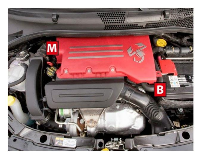
The image above shows the location of the sensors the **Power+ ECM** taps into.
