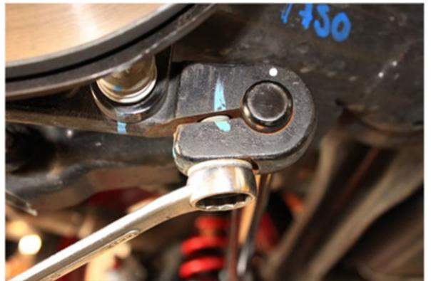
Generously loosen the 21mm Hex bolt on each end of the original torsion bar.
