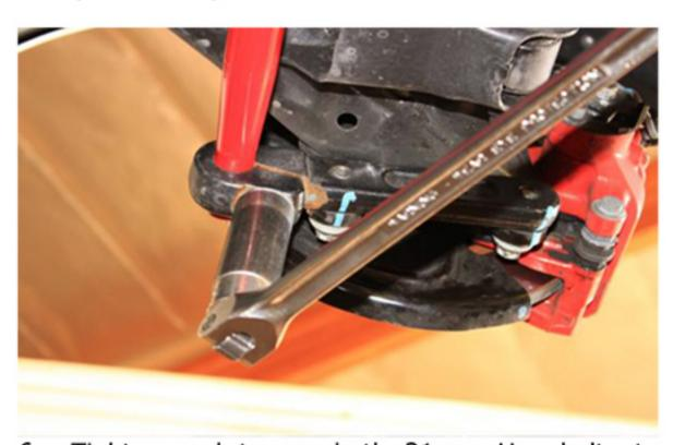
Tighten and torque both 21mm Hex bolts to 176Nm (130 Ft Lbs.)
