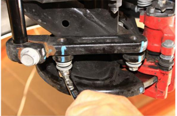
Using E18 Torx wrench unbolt passenger side torsion mounting bracket. Then pull out bar from driver side mount. NOTE: Not the correct tool but a 14mm box end wrench is possible to use. 1 - E18 Torx Wrench (External Torx)
