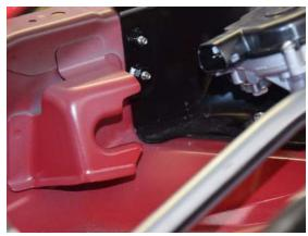
12. Remove the upper firewall cover and remove the 8 10mm bolts.
