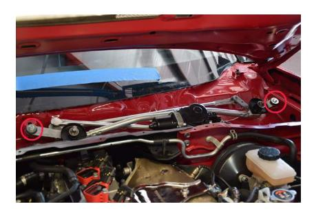
11. Slide the wiper motor assembly towards the center of the vehicle. Be cautious of the windshield. Do not pry towards the windshield.
