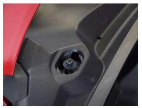
5. Remove the engine bay seal by squeezing the locking tabs from the bottom and gently pulling up on the seal.
