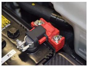
2. Unbolt the 10mm nut and place the positive (red) harness lead to the battery.
