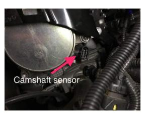
After the Camshaft Sensor is connected to the MAXPower harness, follow the directions of removing the Windshield Wipers and Cowl in reverse order. Be sure to align the windshield wipers to the masking tape used previously.
