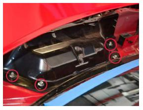
13. Lift from the rear of the cover and tilt forward to remove.
