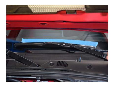
2. Gently pry off nut cover on the windshield wipers by pulling on the edge of it upwards first and with a 14 mm socket, unbolt and remove the windshield wipers.
