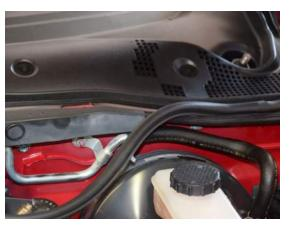
6. Disconnect the windshield washer hose on the passenger side of the vehicle.
