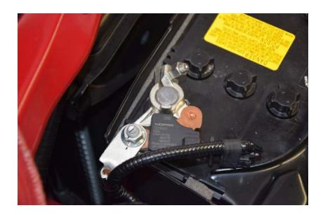
4. Undo the 12mm nut on top of the terminal and place the negative (black) harness lead to the battery.
