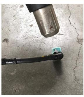
13. Take the push to lock fittings that you removed in step 16 and install them onto 3/8" intake vacuum hose assembly (3 connection) supplied with the MAXFlow intake. Use the following diagram below as a guide. Please note that the larger (purple) push to lock connector is not shown in the photo but is located on the line at the bottom left of the picture.
