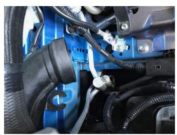
13. Using a long flat head screwdriver reach down behind the ECU mounting bracket on the passenger's side and release the purple locking clip that secures the hard line to the charge pipe on the vehicle. Take the line and set it aside.
