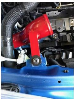
3. Take the 2"-2.5" straight silicone reducer and apply a light coat of silicone spray. Slide the reducer onto the inlet side of the turbo orienting the clamps in such a way so you have access to tighten them. Then take the MAXFlow drivers side pipe and install it on the 2.5" inlet side of the silicone coupler.
