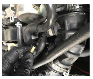
7. Remove the 10mm bolt that secures the molded crankcase tube to the mounting bracket at the front of the motor.
