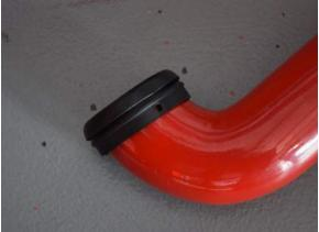
2. Insert the MAXFlow passenger intake tube into the factory inlet duct making sure to slide the hose clamp into place on the inlet duct. Loosely tighten the hose clamp to secure the tube in place aligning the mounting bracket with the hole on the upper radiator core support. Take the supplied M6 washer and slide it onto the factory M6 bolt and hand tighten the bolt in place securing the bracket to the radiator core support.
