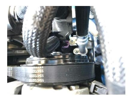
14. Using a regular flathead release the Blue/Green locking clip that secures the hard line to the vacuum box atop the valve cover. Take the line and set it aside.
