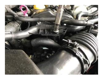
8. Using pliers release the tension from the hose clamp securing Soft Crankcase 3/4" molded line from the vacuum canister on the passenger's side of the engine.
