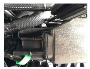
5. Using pliers release the tension from the hose clamp securing the 90-degree vacuum line to the accordion turbo hose. Remove the 90-degree fitting from the accordion pipe. Remove the second vacuum hose that is held to the accordion pipe show below.
