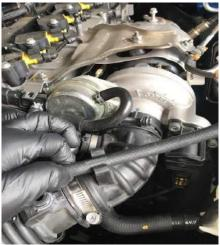
6. Using pliers release the tension from the hose clamp securing manifold pressure sensor vacuum line from the molded crankcase tube. Remove the line from the tube.
