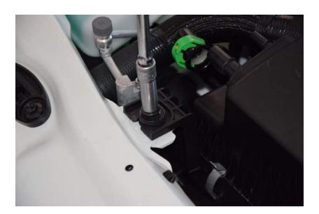
12. Separate the lower airbox inlet duct from the lower airbox assembly. Remove the 10mm nut that secures the lower airbox inlet duct from the box of the car. Remove the rubber isolator from the body this will not be reused.
