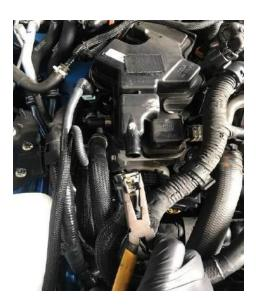
9. Loosen the 8mm clamp that secures the accordion tube to the turbocharger. Remove the entire upper airbox and tubing assembly.
