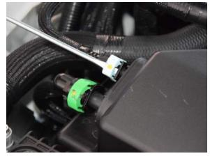
4. Release the two (2) upper airbox spring loaded clips to free the upper airbox from the lower airbox.
