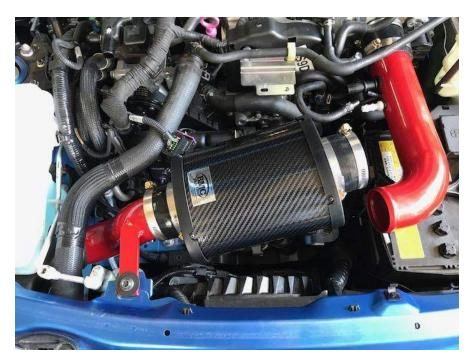
6. Lineup the canister and begin tightening the clamps working from the passenger's side towards the turbo. The hose clamps are 8mm.
